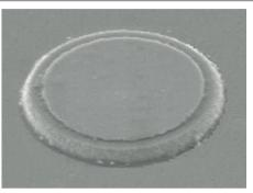
**Fig. 1**| **The first GaN microLED.** Scanning electron microscopy image of one of the first microLEDs, which were based on indium gallium nitride/gallium nitride (InGaN/GaN) quantum wells. The device has a pixel size of 12 μm and p-type nickel/gold (Ni/Au) contact diameter of 10 μm. Figure adapted with permission from *Appl. Phys. Lett.* **76**, 631 (2000), AIP Publishing.
